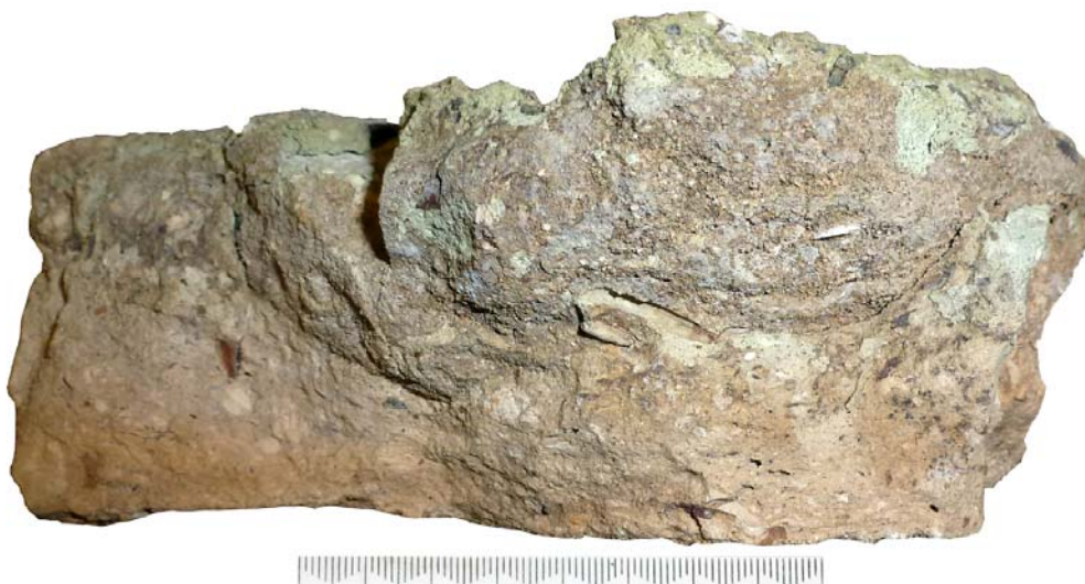
Plate 10. Cross-section of white-firing brick with partial pale green vitrification of the upper surface (1018).
