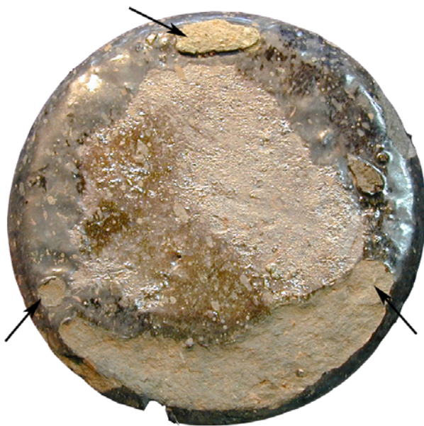
Plate 16. A blackware base showing at least one clay 'bob' and possible locations of two others (arrowed).
